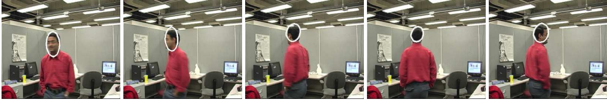
Fig. 1. Motion-Based Particle Filter handles simultaneous jumping and full rotation of the head.
